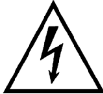
Figure 48: Hazardous Voltage label
