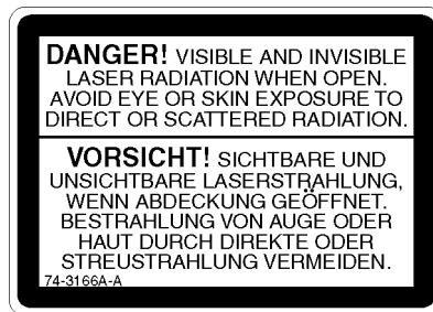
Figure 36: Non-interlocked Panel Danger label
